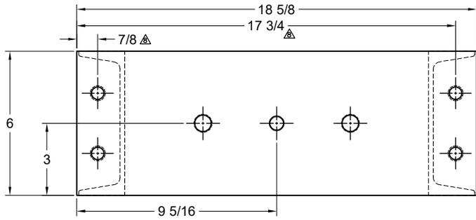
**TYPE M2P-3R SPRING ISOLATORS WITH INTERNAL ADJUSTMENT AND POSITIONING PIN**
